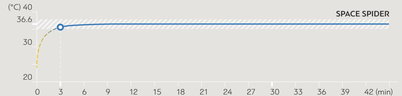
To achieve the very best results, every measurement tool is usually tuned to the conditions of a particular use case. Space Spider, however, keeps its precision in a wide range of temperatures and adjusts to the conditions in only 3 minutes, saving you precious time.
