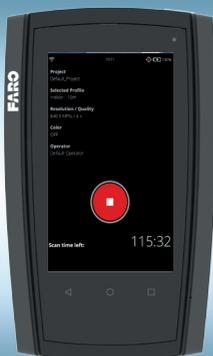
You can abort scanning with the **Stop Scan button** on the display or with the **Start / Stop button** on the scanner.
