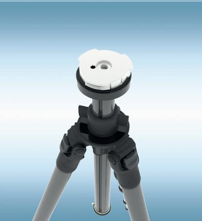
Ensure that the setscrews of the tripod are let-in flush before tightening the part. Mount the counter piece of the Quick Release onto the tripod. Secure the part by tightening the setscrews.
