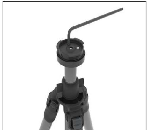
4. Use the S3 hex key to tighten the set screw of the base plate completely against the platform of the tripod.
