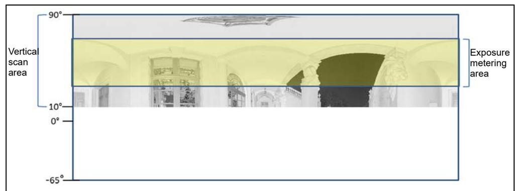
Figure 7-15: Exposure metering area for a limited vertical scan area set to e.g., 10° to 90°
