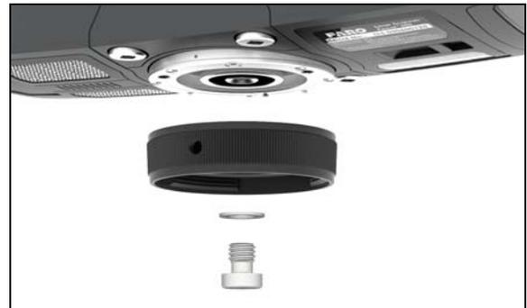
2. Put the S3 hex key (shown here in silver) as an interlock into one of the three openings of the threaded collar. Slightly turn the collar and find a spot where the hex key fits into one of the six openings of the inner ring. Make sure that the hex key actually went into one of the six openings of the inner ring.
