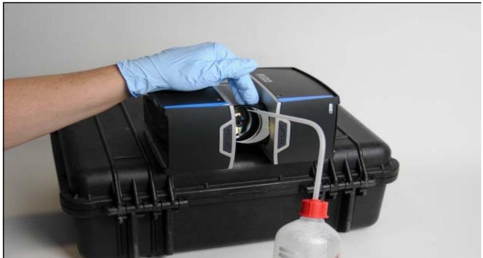
*Figure 9-14: Cleaning mirror module or sensor cover*
