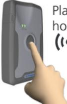
Place the R1 GNSS receiver in pairing mode:
